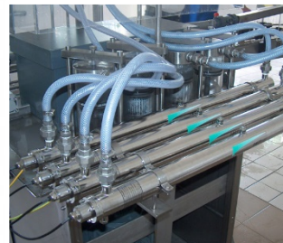
Disinfection of process water in the chemical industry 4x VAP-AW 008 for 1m 3 /h Germany
