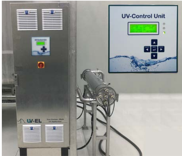
UV-Disinfection System of Sugar with very low UV-Transmission Vietnam
