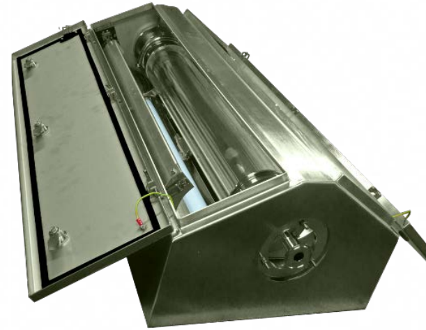
Module for light exposure ( \lambda=320 nm) positive radiation geometry with quartz and filter tube for wavelength selection Germany
