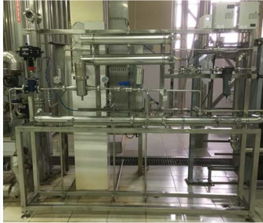
UV systems for air disinfection in a brewery (project with Alpha Corp.) Vietnam
