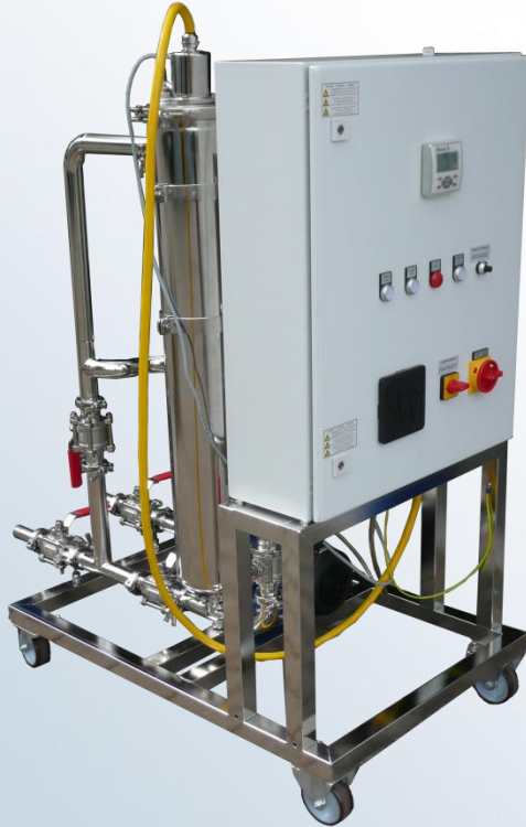
Mobile pilot plant for removal of cyanide in the process water. System has injector for injecting hydrogen peroxide.
